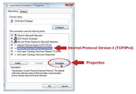
d) In the "General" tab, select "Use the following IP address", and set the IP address as described below.
