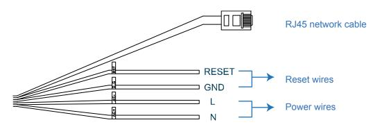
Twist the camera's and power cord's wires together according to the corresponding electrodes (positive to positive, negative to negative, disregarding the ground wire). Then, use the insulation tape to cover the connected wires.
