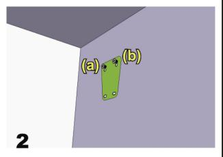
Paste the supplied installation sticker to the location where your camera will be installed. Based on your installation environment, drill a hole in the middle of the sticker for the power and video cable to put through later if necessary.
